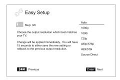
Depending on your selection of "Primary Video Output", the available output resolution selections will differ. For the HDMI 1 and HDMI 2 output, the following output resolutions are available:
